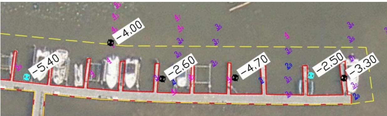
Gator Dredging’s proposal is to dredge all slips to 2.5’ of water at MLT. In addition, to dredge an extra 10’ northward, into the canal. This will provide adequate space to turn vessels and navigate back and forth.
